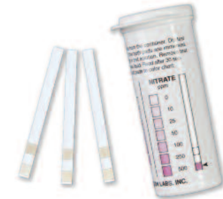
Test Strips- to test nitrate (NO 3 ) content
