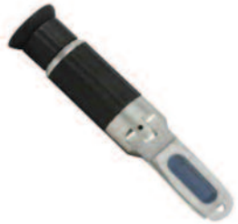
Refractometer- to test sugars
