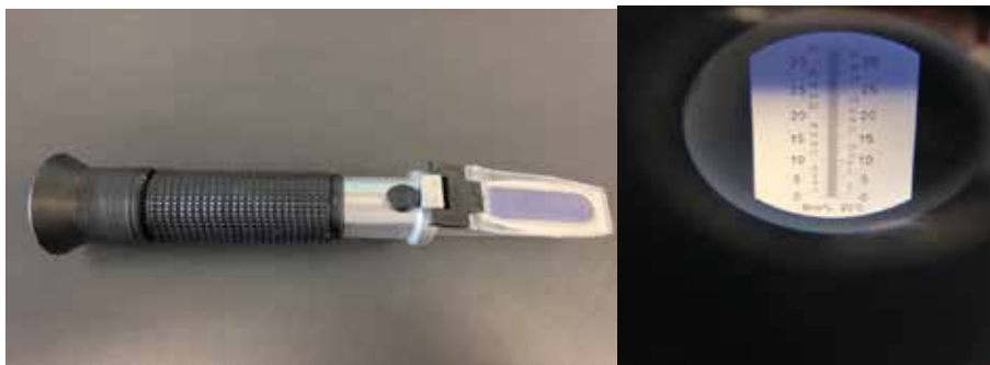
Figure 1. On the left is a Brix refractometer and on the right is the scale observed through the refractometer. When using a refractometer the measurement is recorded at the point where the white and blue colours converge, and for this image the colostrum is estimated to have a Brix value of approximately 25%
