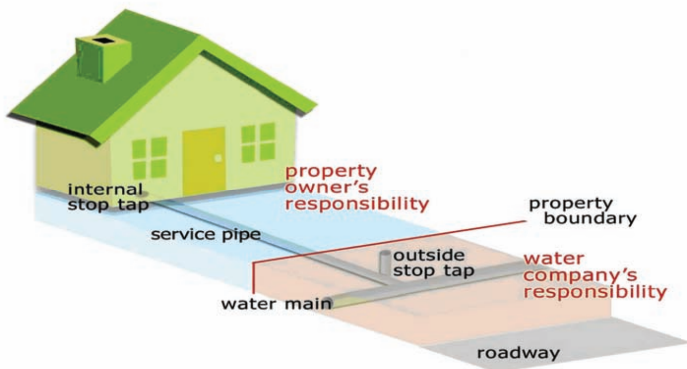
Figure 5.7: Typical Water Supply Arrangements
