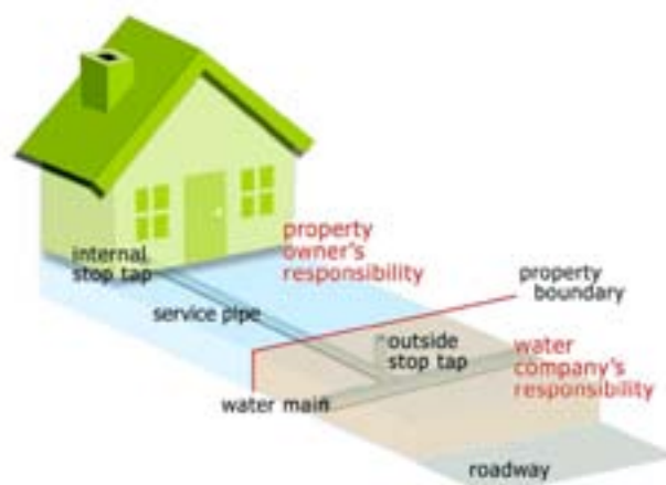
Figure 5.6 Typical Water Supply Arrangements
