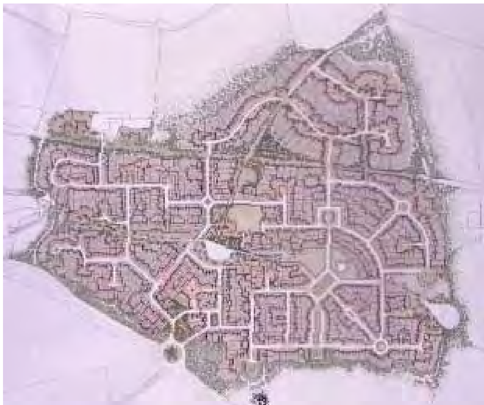
An example of a concept master-plan showing interconnected roads, pedestrian and cycle links, local facilities and open space with variety and distinctiveness displayed in the layout and building forms proposed.
