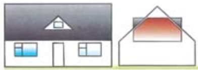
Inappropriate solid: void ratio. Inappropriate proportion to opening in dormer.
