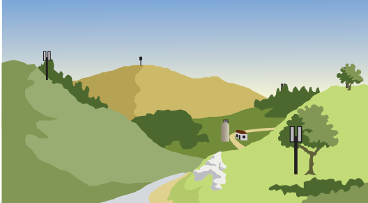
Spreading masts throughout a landscape with many existing landscape elements may have less impact than site or mast sharing
