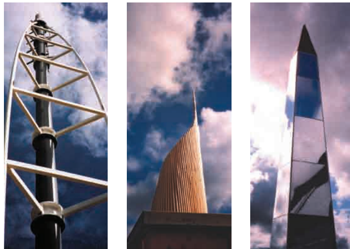
Example of Public works of art which incorporate antennas or complete radio base station.
