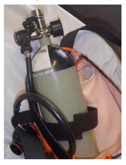
This steel cylinder is the main component of the escape set. This cylinder is steel due to the necessity for the cylinder to resist impact that may occur during work procedures and general underground works. It is pressurised to 220 bar and is 3 litres in size. The bottles are black and white on top to indicate that they contain breathable air. The bottle weighs 3.7 kg when full.
