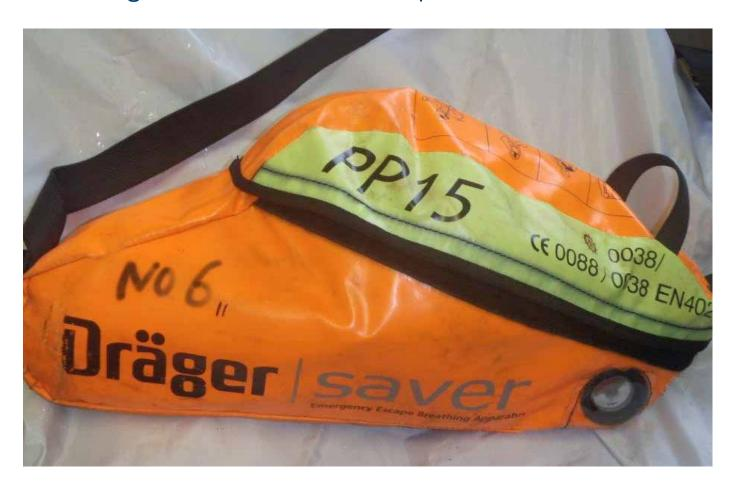
This escape set is classified as breathing apparatus and is intended for use only by those carrying out underground works to escape to a safe environment. The escape set has a limited amount of breathable air depending on the demand of the user. It is anticipated in most situations that on average 15 minutes duration will be afforded to the wearer and this should be factored into planned work activities.
