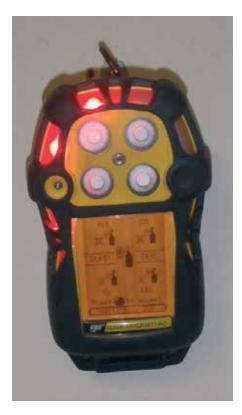
Gas detectors are capable of measuring the concentrations of 4 separate gases:
