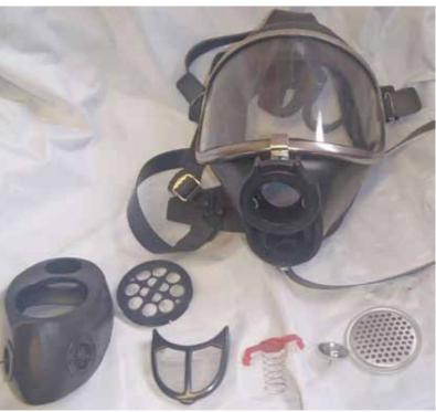
This rescue face mask forms part of the rescue set. The face mask for the rescue set is different from the escape set with 5 strap adjustments as opposed to 2 on the escape set. The head harness is also different as can be seen from the photograph above. The straps are rubber and more durable than the straps in the escape sets. There is a speech diaphragm in the rescue mask but not in the escape set.
