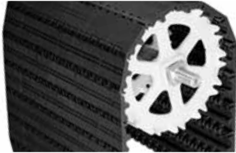
Figure 4.14: Illustration of screen mesh rotating vertically around polymer sprockets (courtesy of Hydrolox).
