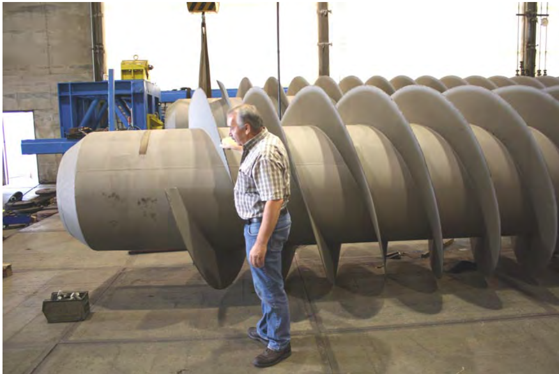
Figure F5.6. Archimedes screw runners at the Landustrie factory for refurbishment. These are about 1.8 m diameter, but they have been made up to 5 m in diameter and 25 m in length.
