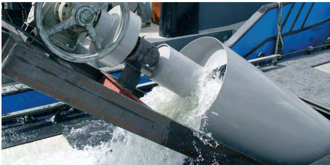
Figure F5.9. Top end of an Archimedes Screw pump with a fixed tube or shroud throughout its length. Photograph courtesy of Fish Flow Innovations.
