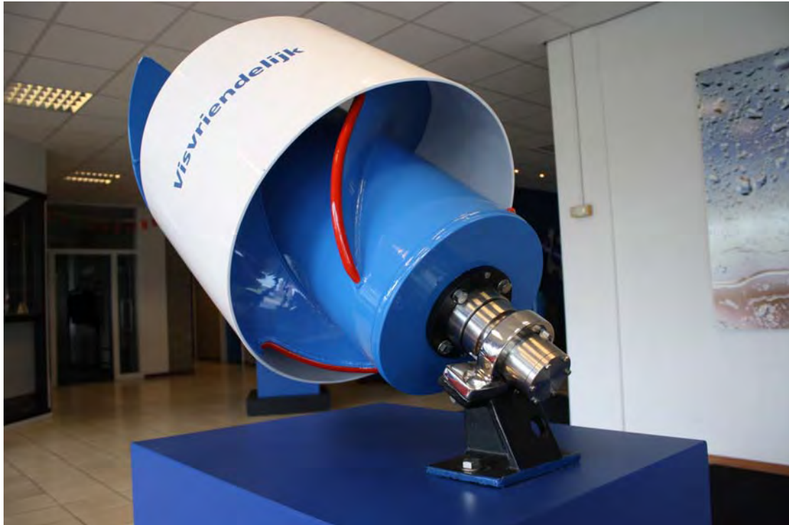
Figure F5.7. Lower end of a “fish-friendly” Landy Archimedes screw pump, showing the specially-designed leading edges (red) and the rotating shroud (the grey structure with the word “visvriendelijk”). Photograph courtesy of Landindustrie Sneek BV.
