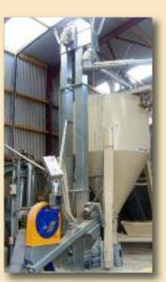
mixer allows four times the amount of feed to be mixed in the same amount of time. In the 12 months since the installation of the new hammer mill and mixer the producer has seen a reduction in his electricity bill despite over twice as much pig feed now being mixed.
