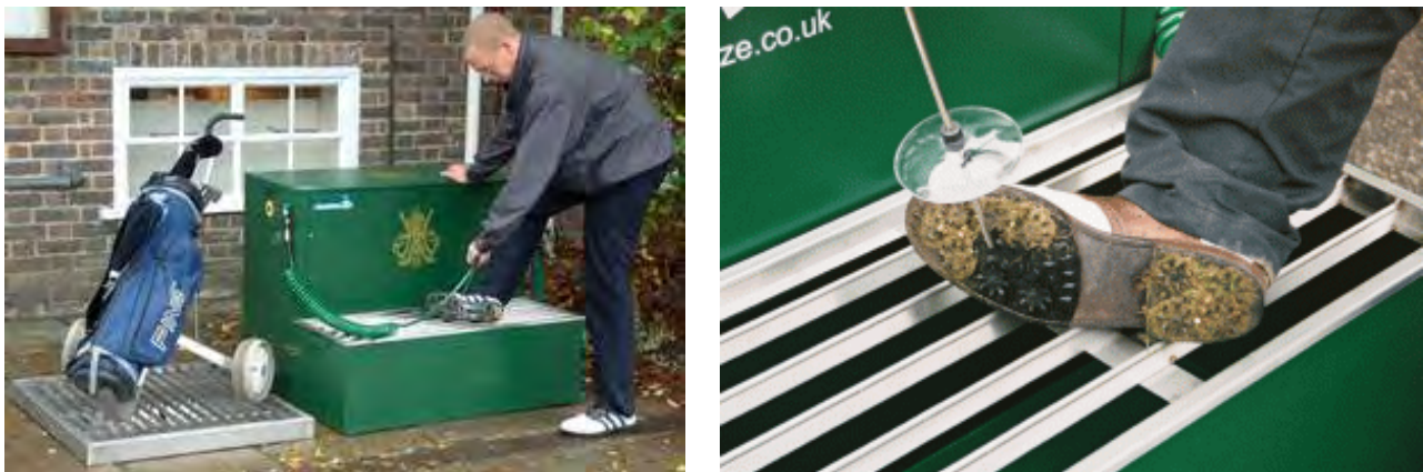
Figure 4. Typical air blower for cleaning shoes and equipment. Air jets transfer soil and plant material from shoes etc. into a collection bin for subsequent removal and disposal.
