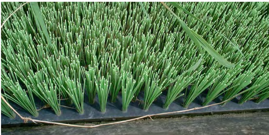
Figure 5.1 Bristle substrate with nylon bristles fixed to a polypropylene sheet
