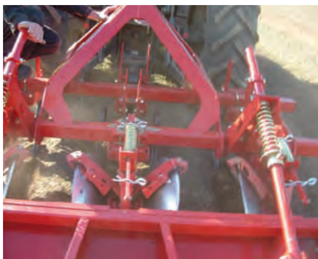
Loosening compaction on the shoulder of the ridge using tines mounted on the front of a rotary tiller also allows greater water infiltration and crop rooting.
