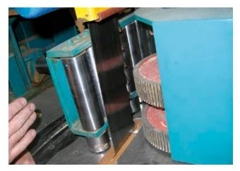
Figure 10 Single-cut band re-saw – details of feed rollers
