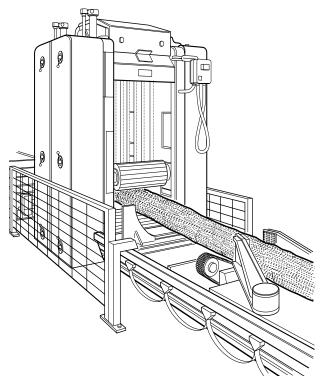
Figure 12 Frame saw (barrier along feed track not shown)
