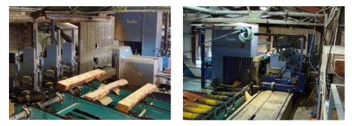
Figure 8 A reciprocating carriage log band saw – feed on to carriage and carriage approach to band saw
