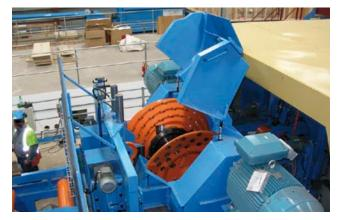
Figure 27 Chipper/reducer and covers
