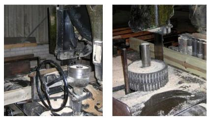
Figure 3 Stand-alone band saw with manual feed and optional power feed without guard fitted
