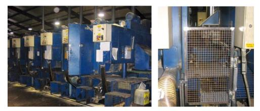
Figure 6 Older mechanically-fed six-in-line horizontal band saws with retrofitted interlocked hinged gate between machines
