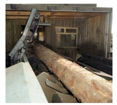
Figure 24 Butt reducer
