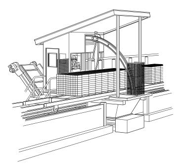
Figure 20 Static cross-cut chainsaw
