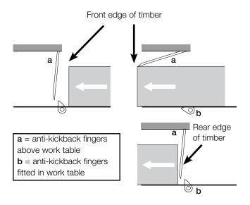
Figure 16 Anti-kickback fingers on multi-rip saws
