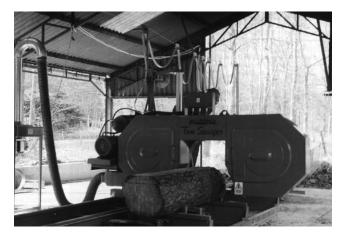
Figure 9 Moving head-rig log band saws
