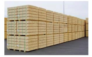
Figure 34 Well-built stacks of banded sawn timber packs
