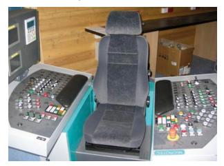
Figure 31 Automated sawmill control room
