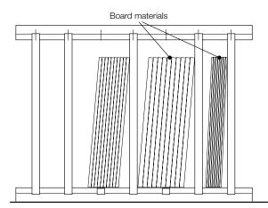
Figure 35 Wooden sheets/boards placed in a purpose-designed storage rack
