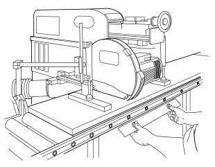
Figure 17 Semi-automatic horizontal cross-cut saw
