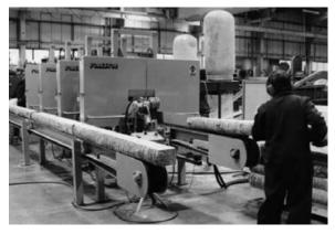
Figure 4b Hand-fed multi-cut band re-saws
