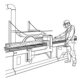
Figure 13 Travelling table circular log saw
