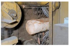
Figure 21 Through-feed debarker (guards not shown)
