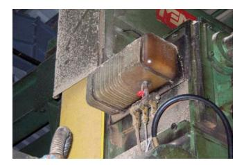
Figure 2 Automatic lubrication system
