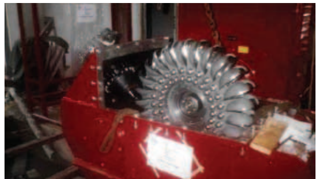
A Pelton Turbine with upper casing removed
