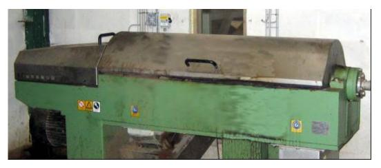
Figure 2. Decanting centrifuge.
