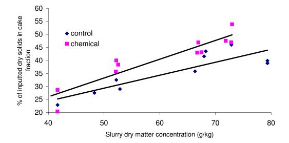
**Figure 9.** Relationship between cattle slurry dry matter concentration and the percentage of dry solids partitioned to the separated solid fraction with the brushed screen separator.
