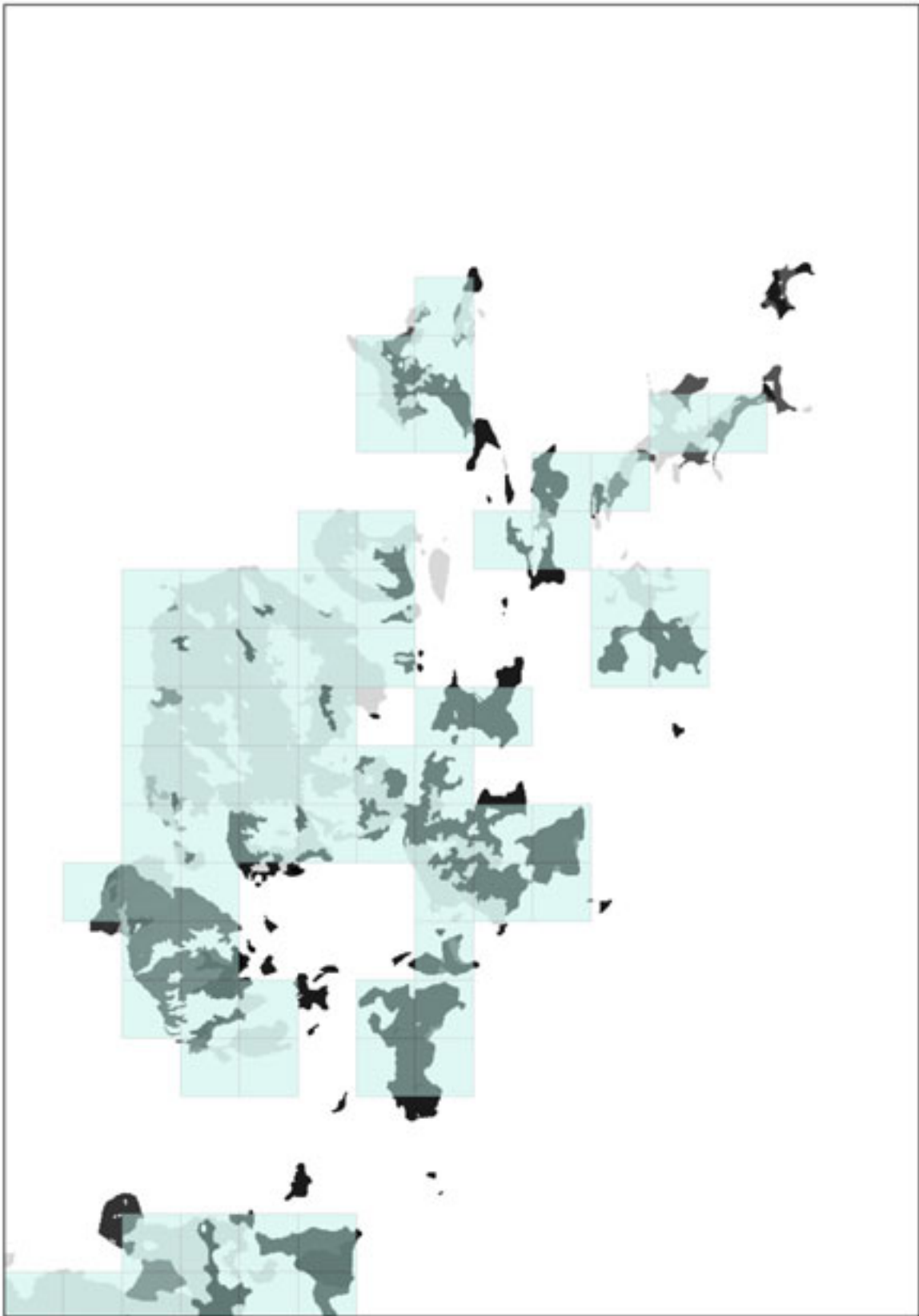
Figure 3.6 Example of mismatch in coverage between 5km climate and 100m soils map grid cells.
