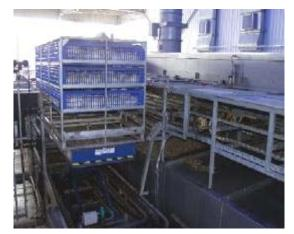
Diagram 15: Crates being loaded into a controlled atmosphere stunner
