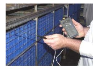
Diagram 6: A portable temperature and humidity sensor being used in the lairage
