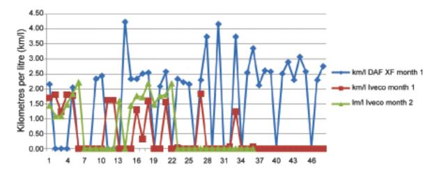
Figure 3: Km/l of Daf XF (general) vs Iveco Stralis (timber).
