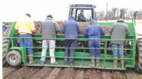
Wexgen Planter requires five operators and the driver.
