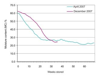
Figure 4: Time required for drying to 30% moisture content, relative to the start month of the storage trial.
