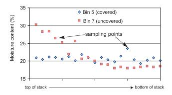
Figure 6: Moisture content of the samples was dependent on position in the stack (covered bin 5 is compared to the uncovered bin 7).
