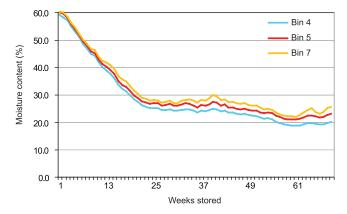
Figure 5: Drying rates of bin 4 (covered sides and top), 5 (covered top) and 7 (uncovered) decreasing with less cover of stacks.
