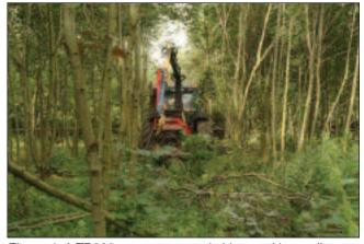
Figure 4: A TP280 tractor-mounted chipper with a trailer attached to collect the chips.
