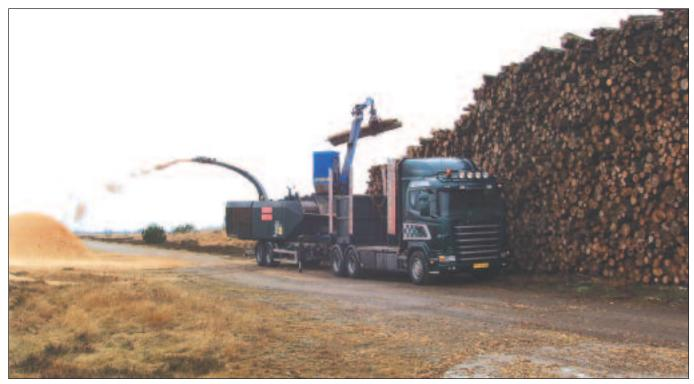
A truck chipper processing a pile of 3 m pulpwood. Note the stacking height.
