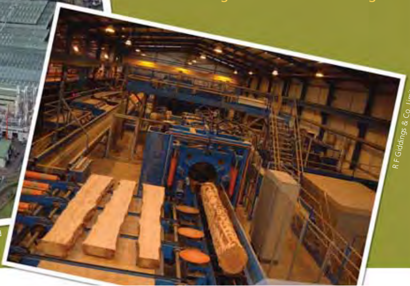
Below: Giddings – 3D Log scanner – maximising the value from each log
