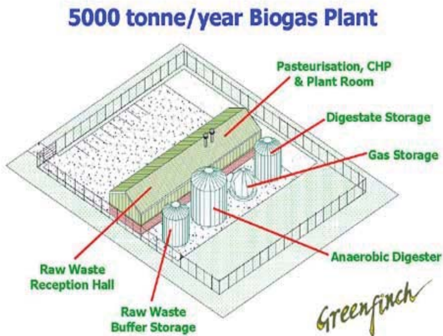
Figure 28 Schematic of Greenfinch plant http://www.greenfinch.co.uk/ Greenfinch Ltd. (2005). Business Park, Coder Road, Ludlow, Shropshire, SY8 1XE. Tel; 01584 877687.
