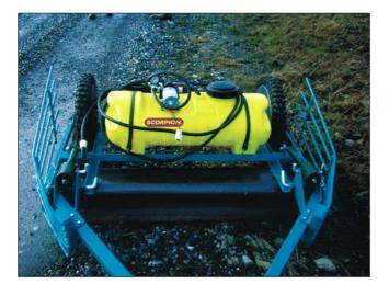
**Photo 10**: The weed-wiper machine can be used to control vegetation on cutaway where mowing is not feasible.
